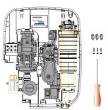
Fit Rubber Feet and fix appliance to wall.
