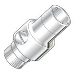
**DCV-H:** An outlet double check valve, designed to prevent the backflow or backsiphonage of potentially contaminated water, through shower controls which are fitted with a flexible hose as part of the outlet shower fitting. Available as an optional accessory from your Kohler Mira stockists.
