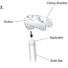
Depress button **FULLY** and assemble Clamp Bracket. Release button and remove Applicator.
