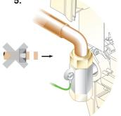
For rear inlet, use soldered elbow. Do not trap green wire.
