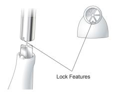
Fit both the top and bottom Supports. Make sure the slots are aligned to fit fully home. 5.
