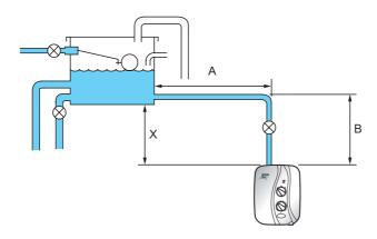
**Example!** The example below is based on the diagram above with 15 mm pipework, A = 1.5 m, B = 0.75 m.
