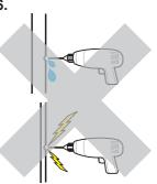
CAUTION! Do not drill into buried cables or pipes.
