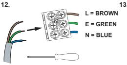
Firmly connect the conductors. Do not exert strain on the terminal block.
