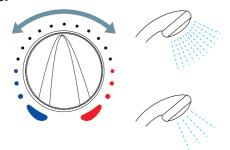
Adjust temperature as required. Flow rate will adjust automatically.
