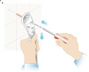
First fix the bottom Slide Bar Support and fully tighten the screw\*. Then fix the top Slide Bar support whilst pressing it down, to keep the whole assembly together.
