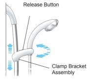
Depress the release button and slide the Clamp Bracket assembly to the required position. 2.
