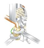
Connect supply pipe. Do not overtighten!
