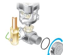
Press down on the filter cover and turn anti-clockwise to release.
